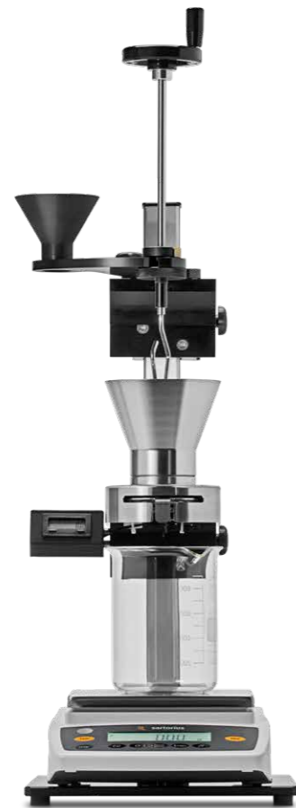
Flow through an orifice — with funnel
