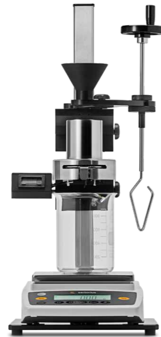
Flow through an orifice — with cylinder
