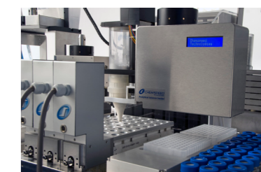
Overhead gravimetric dispensing of solids directly into parallel synthesis reactor array
