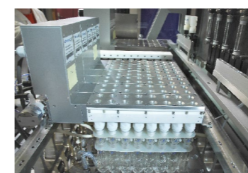
Example of a tray configuration with reactors for impregnation solutions, reactors for impregnations, liquid handling unit, gravimetric powder and extrudate dispensing unit, a variety of racks, and much more...
