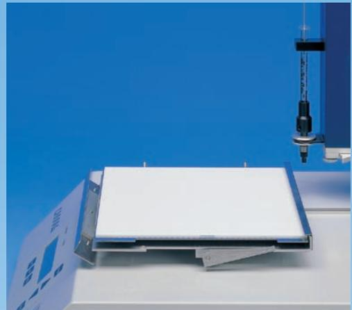
The self-adjusting object support enables application onto objects of variable thickness (up to 4 mm) without any adjustment to the spray nozzle. This makes changing between conventional TLC and HPTLC layers, on glass plates and sheets, preparative layers and very thin objects such as membranes easy. The support accommodates objects up to 20 × 20 cm.
