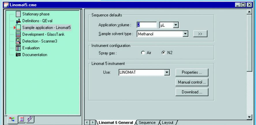
In the tab "Sequence" all parameters relevant to the actual sample application, such as designation, volume and position are entered.
