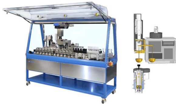
Figure 4 – Formax, Chemspeed Automated Formulation Workstation and Gravimetric dispense WHILE processing
